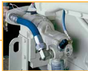
The 150BMGE21RH-6 starters are shown mounted on a Cummins KTA14-M3 and KTA19-M4I.
